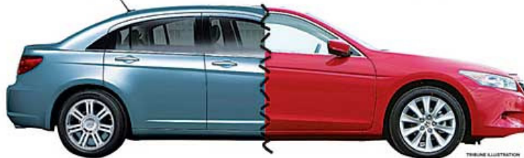
The 'clip job': welding together the undamaged halves of two cars.
